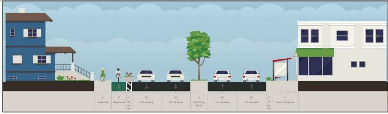
Using approximate measurments: A potential Complete Streets retrofit on Norwood could include buffered bike lanes, a transit shelter, wider sidewalks, and a center median
