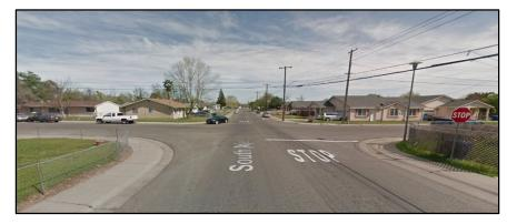
amenities, these streets are characterized by a lack of bike lanes, sharrows, or striped shoulders, intermittent ADA accessibility, attached sidewalks, utility poles within sidewalks, narrow corners with wide turning radii, and no traffic calming features other than on-street parking.
